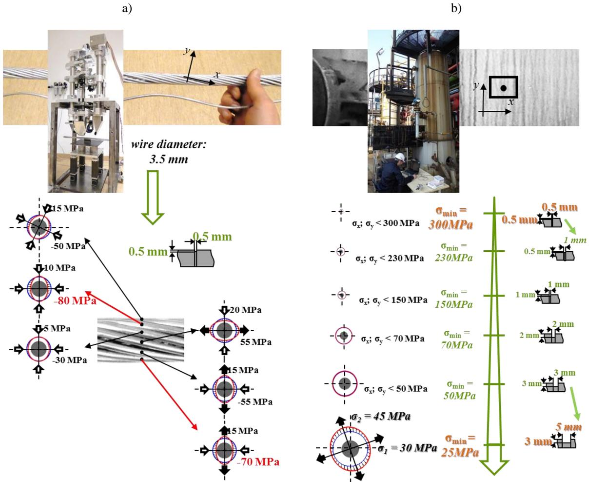
Fig. 4. (a) Residual stress in wires of twisted multicore aluminum cable: measured with extremely small blind-hole-drilling; (b) Residual stress in pressure vessel (after long term use): measured with controlled and minimized incremental blind-hole-drilling
