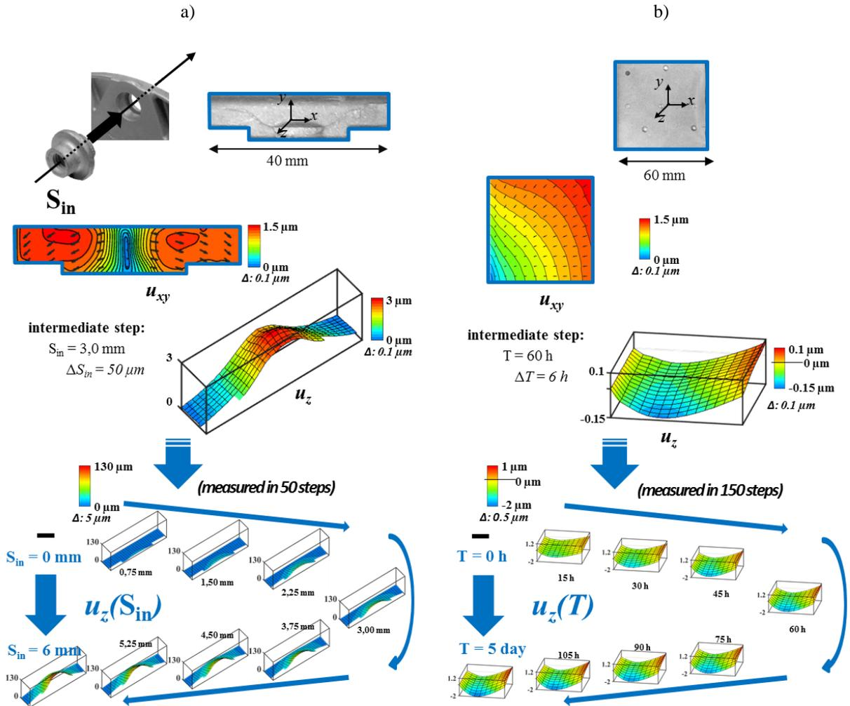
Fig. 2. (a) The complete deformation process of pressing of aluminum sleeve and a steel pin into each other: *up to extended measuring range*; (b) The complete deformation process of self-shrinkage of injection molded plastic plate: *long term monitoring*
