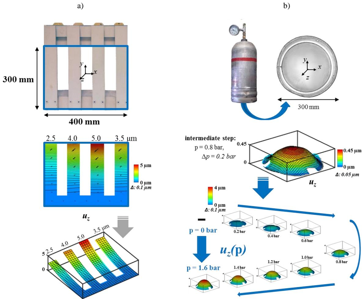
Fig. 1. (a) Large field of view: deformation of cantilever beams at micrometer screw controlled loading at the top; (b) Large field of view: The complete deformation process of bulging of a pressure vessel bottom
