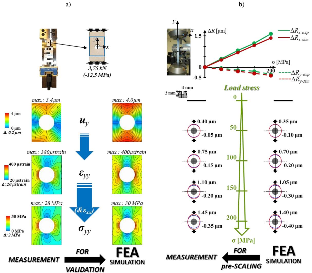
Fig. 6. (a) Deformation measurement for validation of simulation; (b) Hole-drilling stress-relief deformation in simulation for pre-scaling of stress measurement.
