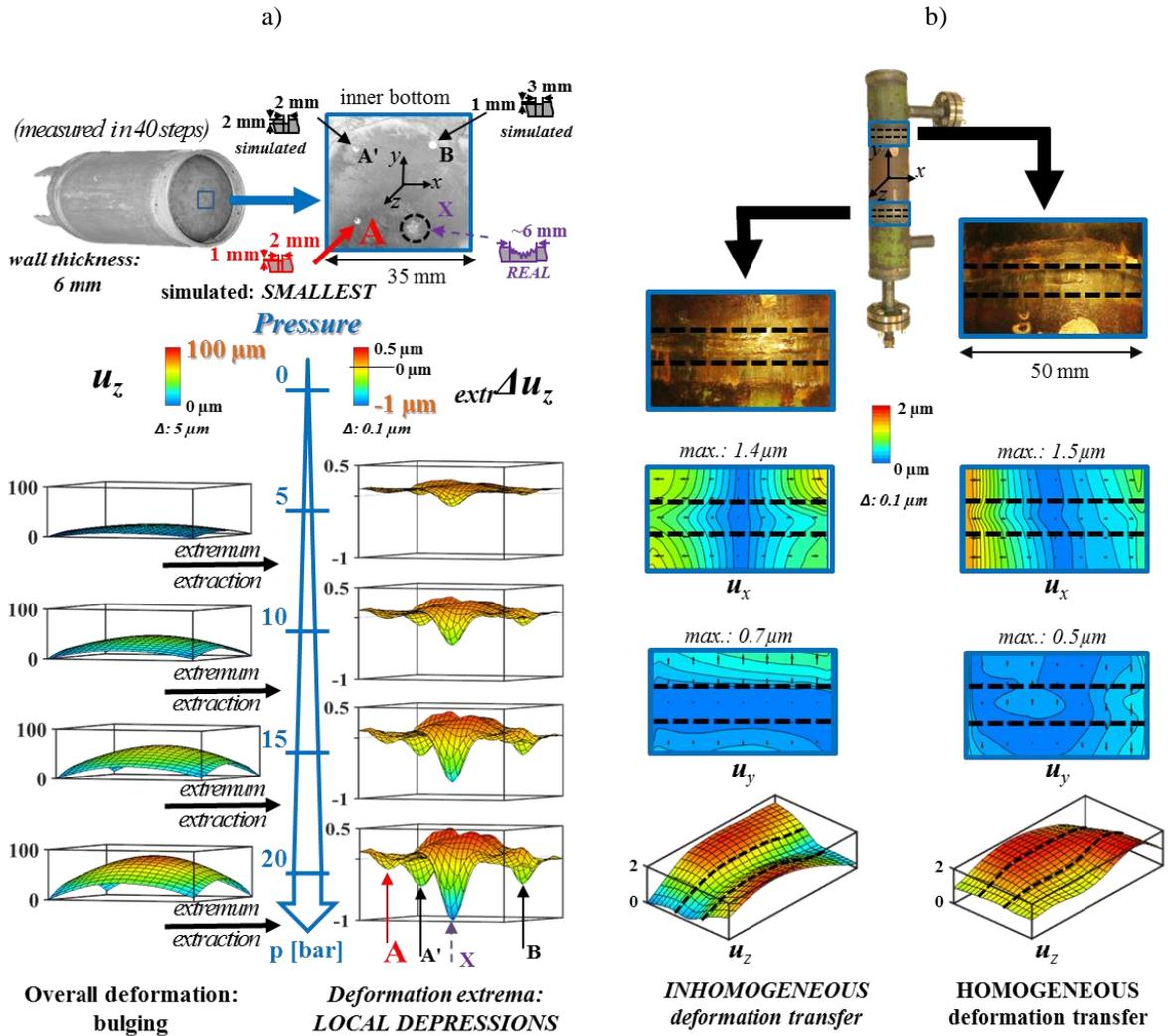
Fig. 3. (a) Monitoring of extra-large pressure deformation and extraction of tiny deformation extrema on it: at corroded pressure vessel bottom; (b) 3D deformation of different welds for comparison with surroundings: to control their deformation transfer property
