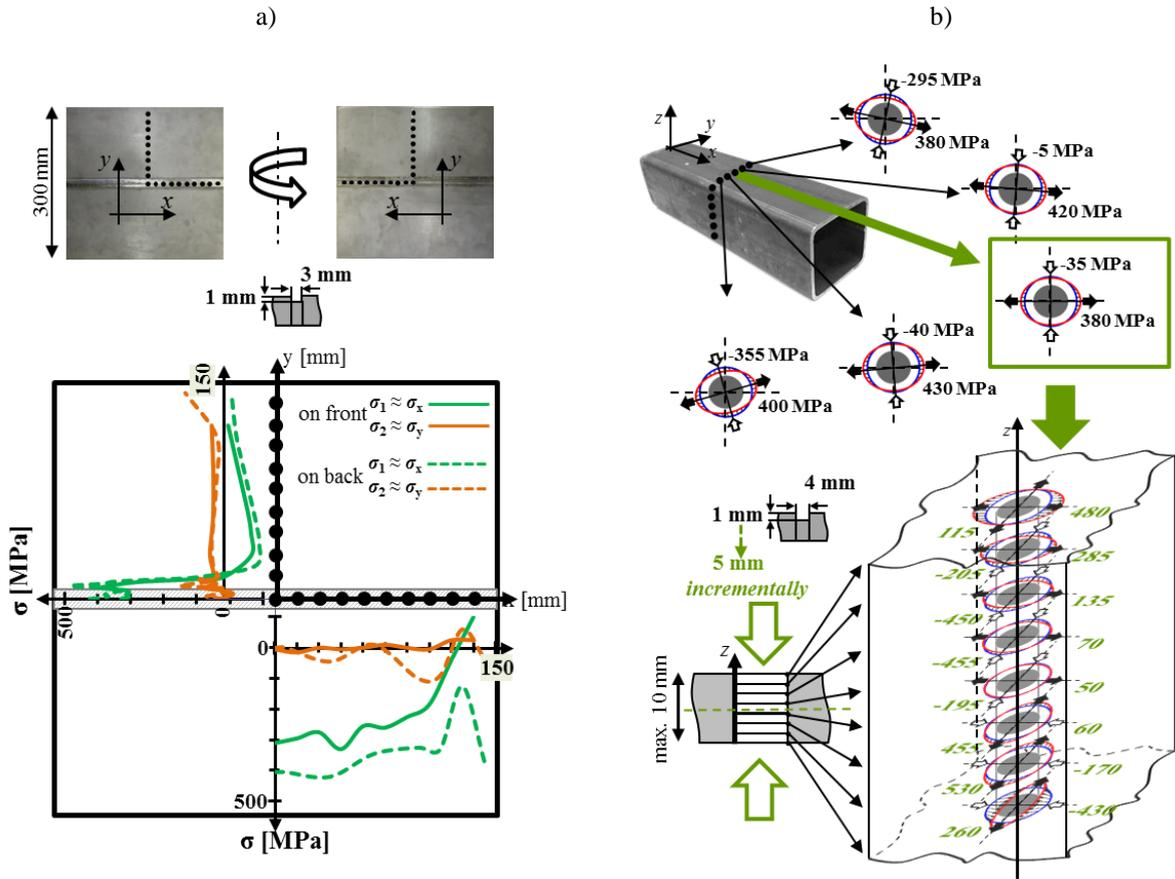
Fig. 5. (a) Residual stress distribution along the weld and along a perpendicular line; (b) Residual stress distribution in welded hollow section along a contour-line and through full depth.
